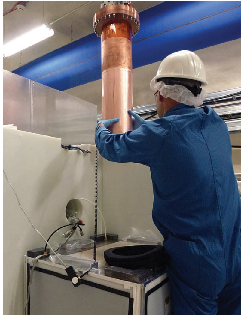
DAMIC installation at SNOLAB: the copper vacuum vessel being inserted in the lead shield
